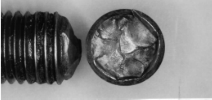
Figure 5. Fatigue fracture, second cap screw. A detailed view of the wear on the edge of the cap screw head is shown at the bottom of the figure.
