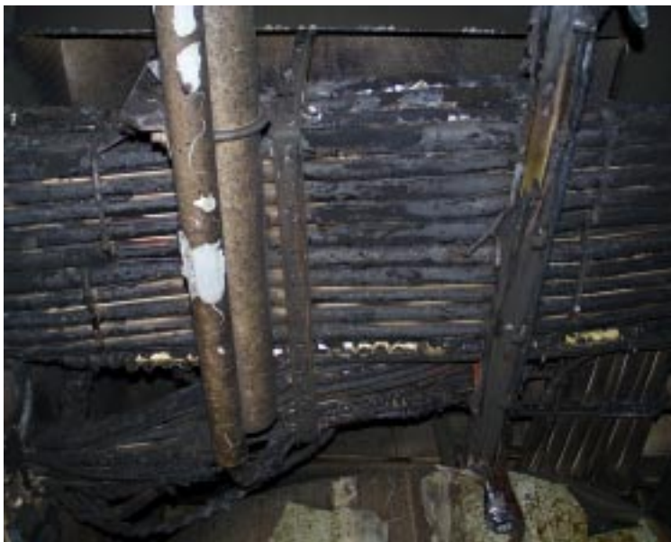
FIGURE 4 Fire damage to deckhead cables and fittings
