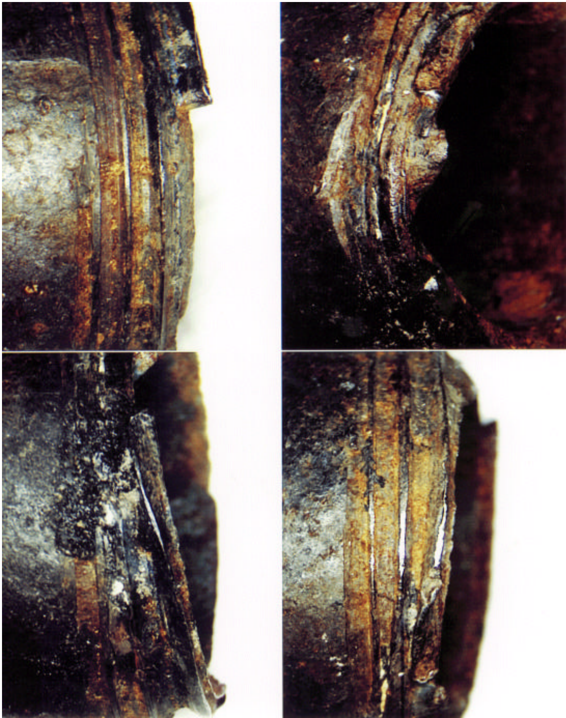
Figure 39 90° rotational view of the condition of the pipe threads on the one inch pipe (A1). MAGNIFICATION: 5X
