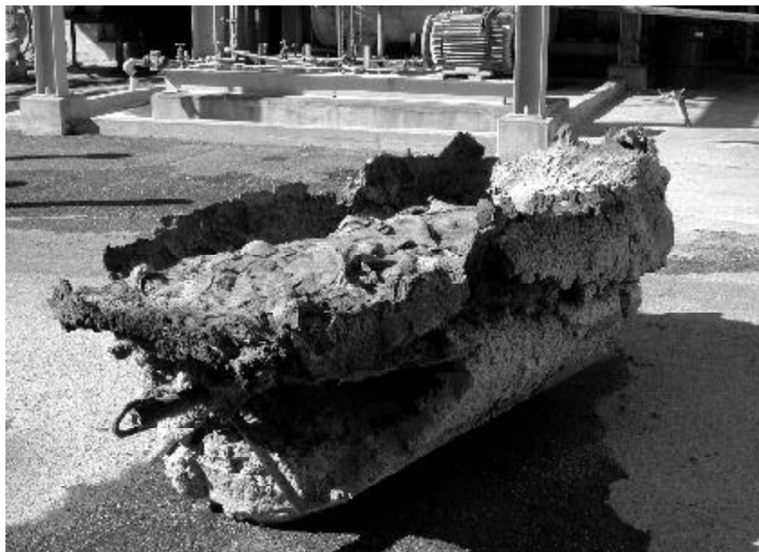
Figure A-6. Material extracted from polymer catch tank on March 11, prior to incident.
