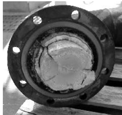
Figure A-4. Vent line obstructed by polymer layers.
