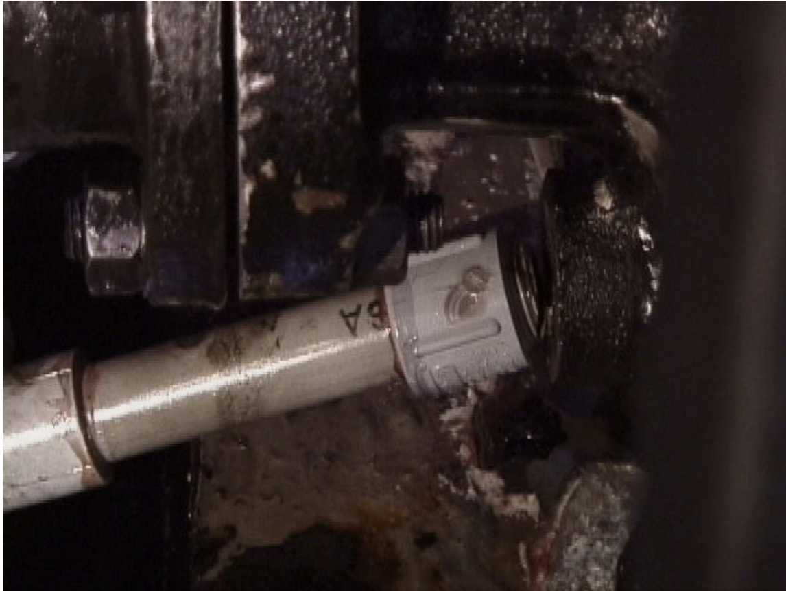
Fractured drain line. Notice line still connected by 20% of lower section.
