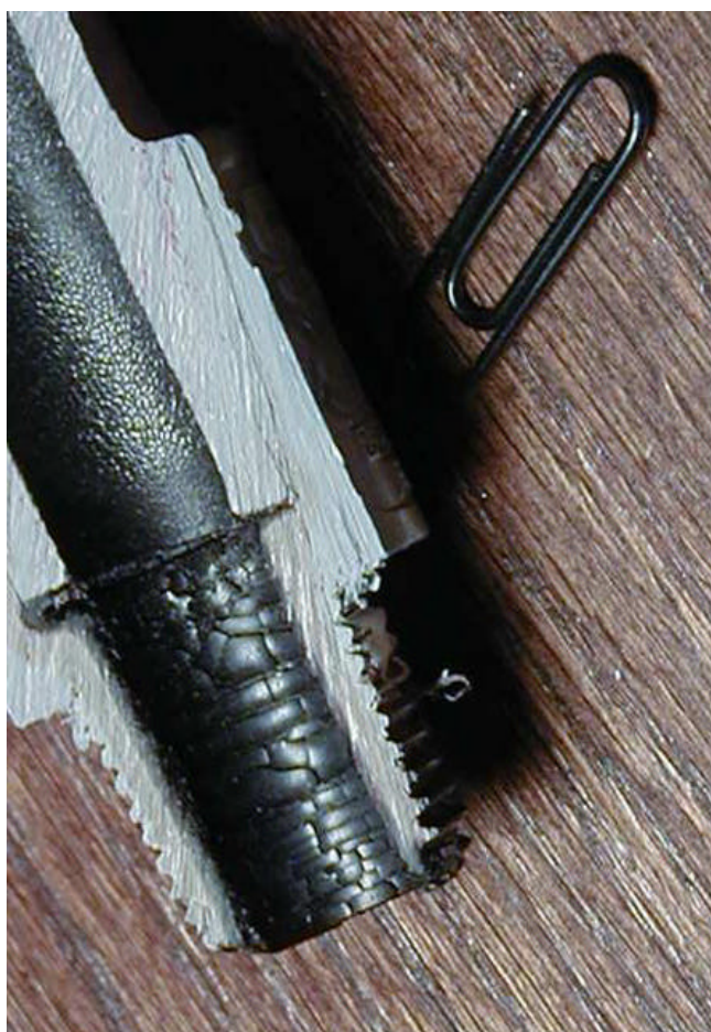
Figure 8. Degraded CPVC piping section, removed from same service in 9/97. (Courtesy of Waste Management Federal Services of Hanford, Inc.)
