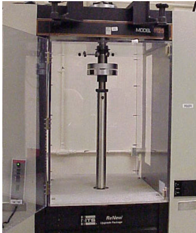
Figure 34. Model 1125 Sintech/MTS Tensile Testing Machine w/test sample
