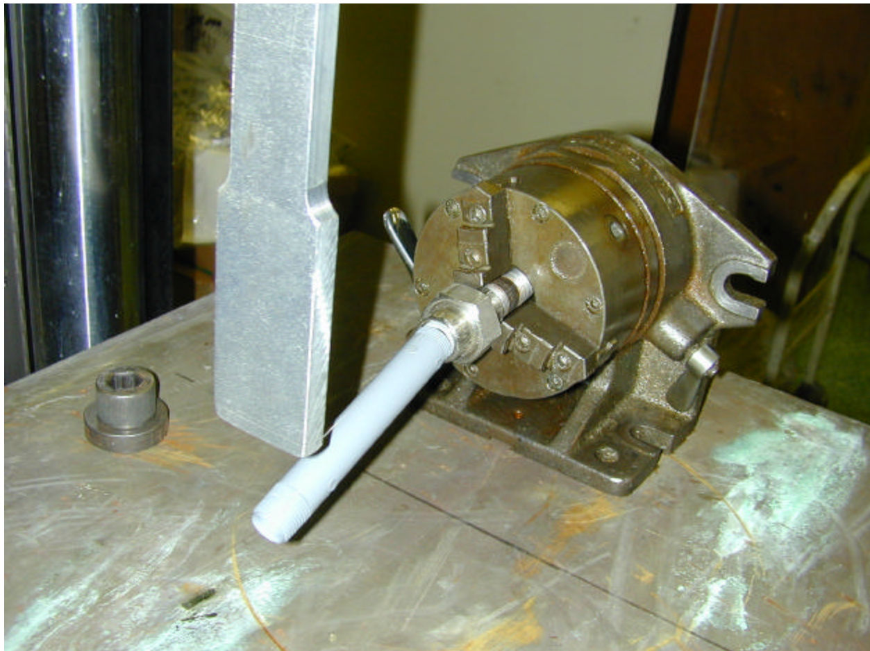
Figure 36. Bend testing of 6" Sch.80 CPVC pipe nipple (non-degraded)
