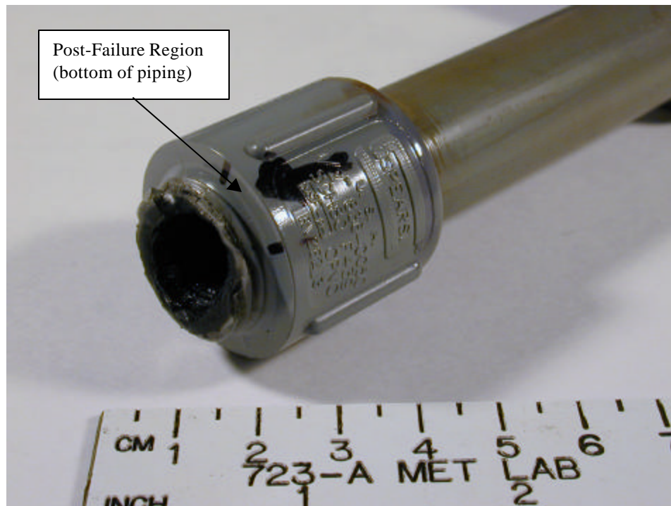
Figure 13. Failed 1/2" diameter Sch. 80 CPVC fitting, Spears Mfg. Part#836-005C
