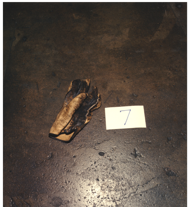
Standard Work Glove Burned from Explosion/Fire
