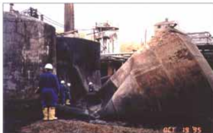
C. Tank 488, after explosion.
