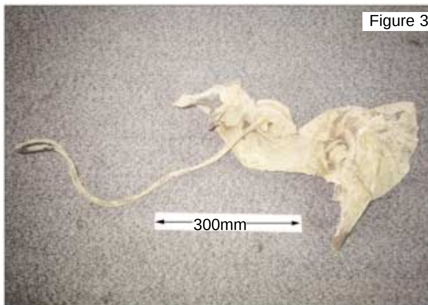
Cylinder top, with element of immersion heater
