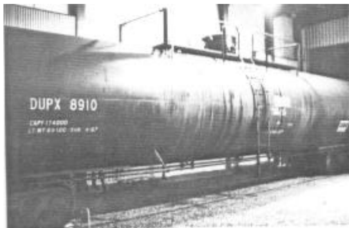
Sodium tank cars are loaded in a dry environment.
