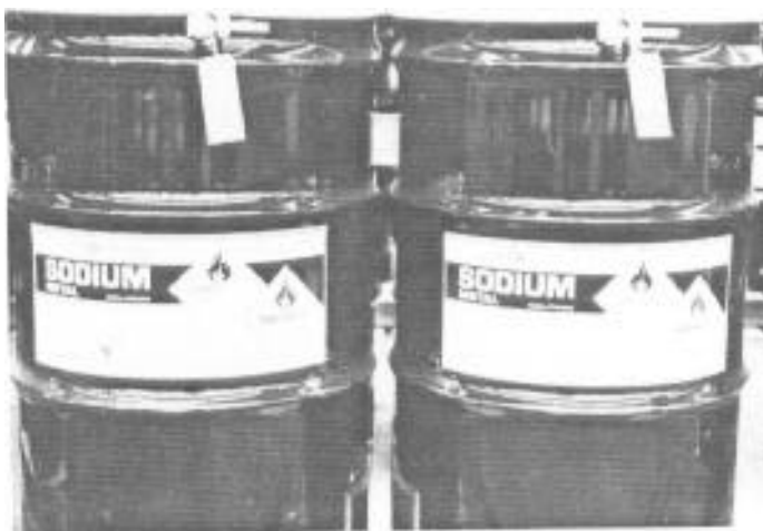
Sodium bricks are sealed in airtight drums for delivery.
